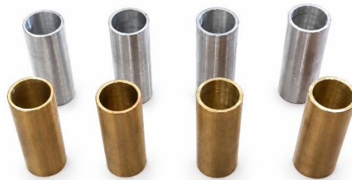
Figure 7. Manufactured expansion samples.
